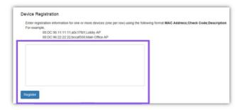
**Note:** The 'check code' of the AP can be found on the device label at the bottom of the AP. Or, access the AP's user interface and find it under the *Management* > *Controller Settings*. Contact your local dealer if you are having problems locating the check code.
